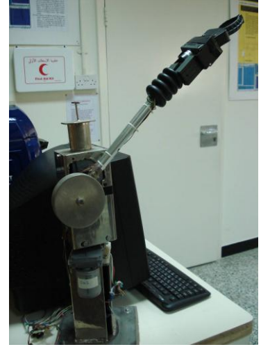
Fig. 1: (Left): Integrating ANN with a two links robotics arm, (UoB-Arm), refer to Mattar [9] for details. (Right): UoB-Arm, a two links robotic manipulator with known dynamics, Including uncertainties.
